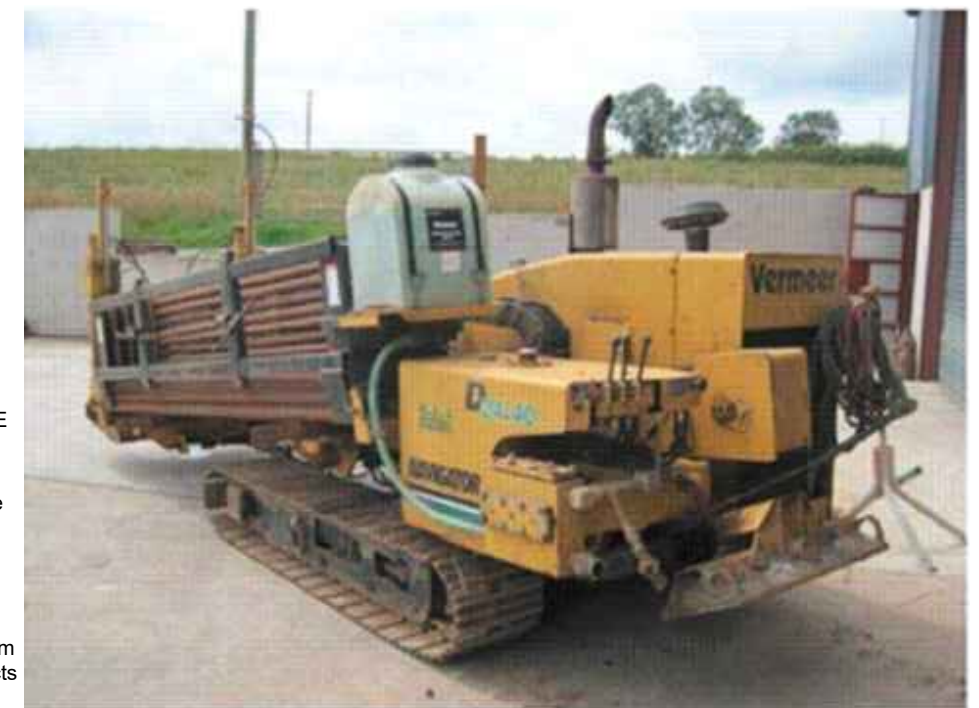
Directional Drilling Rig
